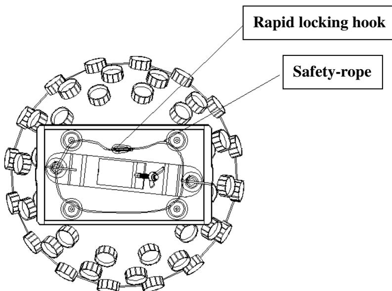
Insert the quick-lock fasteners of the first holder into the respective holes on the base of the product. Tighten the quick-lock fasteners fully clockwise. The mounting bracket can then be attached to a stand, trussing or lighting bar securely. Be sure to use a safety chain which connects through the lug with the hole in it on the base and around the trussing or bar on which the product is being mounted.
