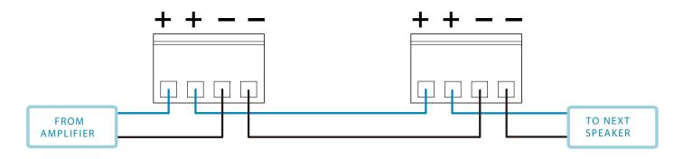
Select the wattage tap by dividing the amplifier's maximum available power by the number of speakers to be connected. Always select the next lower wattage tap. For example...
