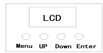
Menu – Move up a level. Up – Move selection up one item. Down – Move selection down one item. Enter – Select / Move down a level.
